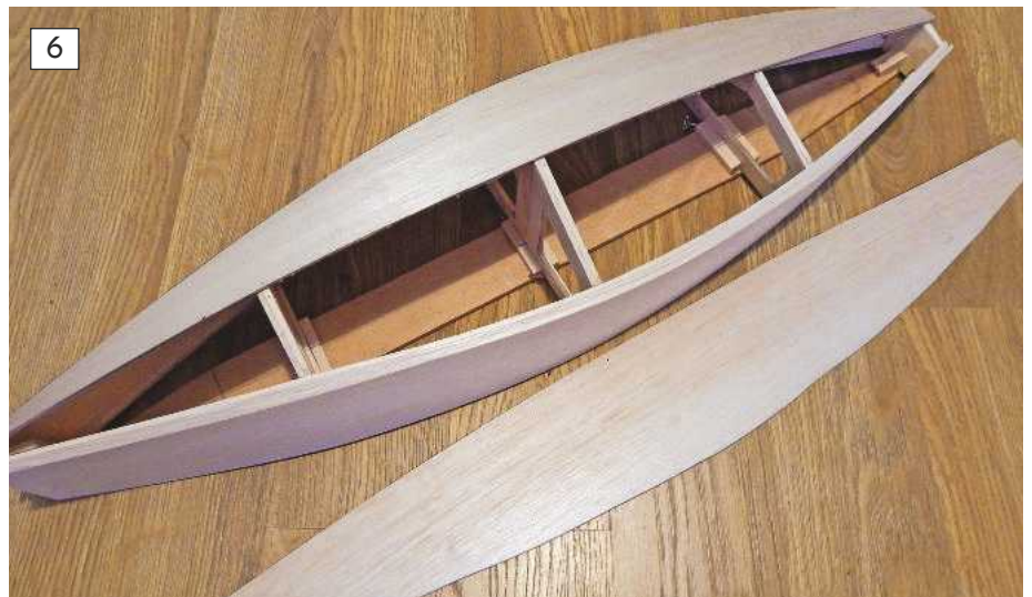
6. Don't rush this bit. Time and patience will pay dividends with a perfectly-fitting bottom skin and centre joint.
