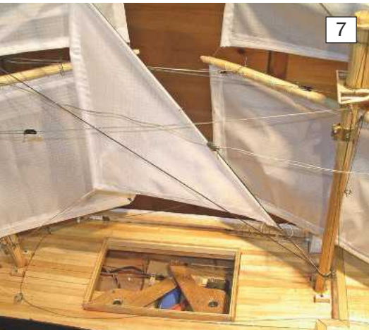
7. An overlapping servo sail arm installation. Please note the relationship of the angles between these arms and the yards, remembering that the sail arm on the right controls the yard on the left and vice versa.
