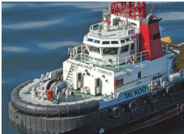
BELOW: Bow view showing the forward ship-handling winch. Note the two air conditioning boxes and bridge roof detail.
