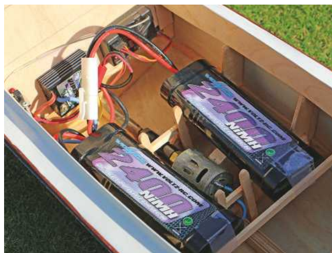
ABOVE: One of these 2400mAh NiMH packs will run the boat for longer than I ever need to sail her. The other is used purely as useful ballast.
