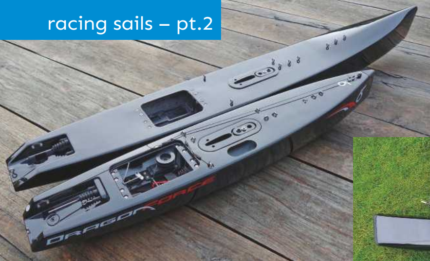
ABOVE: December 2014. The final DragonFlite 95 prototype hull, beautifully built by Alex Cory. The deck design was not finalised at this stage, the final profile featured more detailing to provide rigidity.
