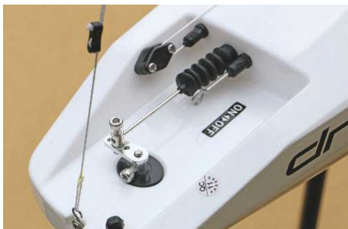
The DF95 cockpit with sheltered on / off switch.
