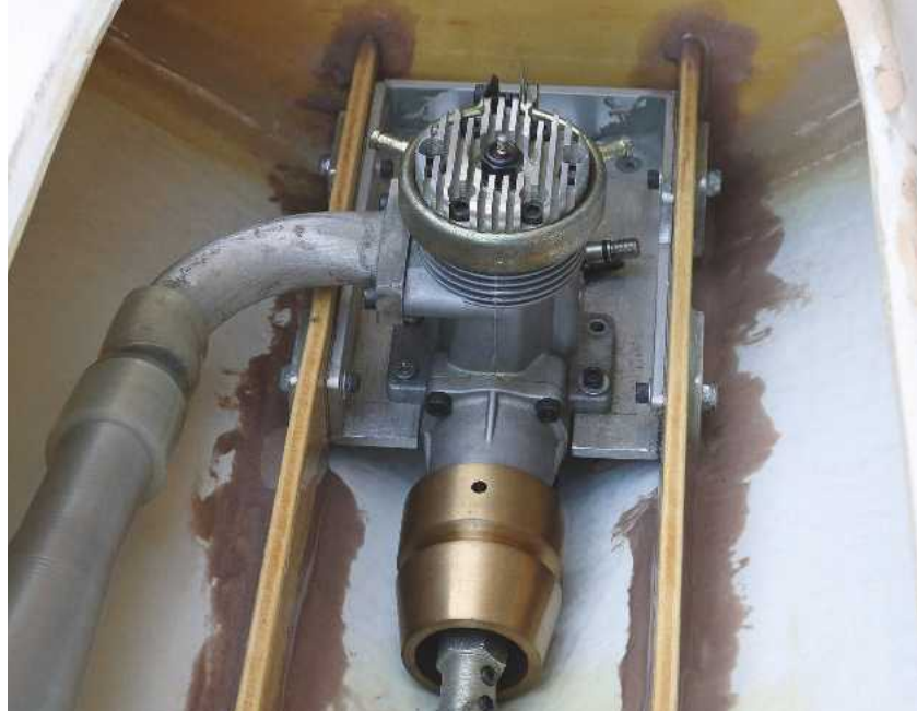
RIGHT: An aircraft engine with clamp-on water-cooling collar and custom-made flywheel in a racing boat (J. Boys).
