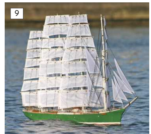
One of the reasons for separating the sail control between the masts. Here, the foremast yards of Peter Rickmers are taken aback during tacking, just like the real ship.
