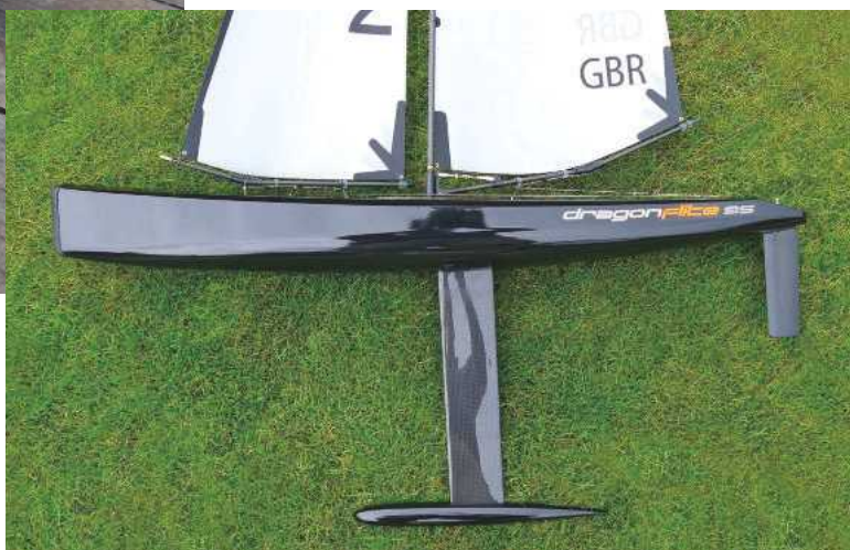
RIGHT: August 2015. The first sample production boat. They sent over two samples, one white, one black. One feature that changed before the boat went into production was the keel. Originally it was to be extruded aluminium but the profile was not possible to extrude to the accuracy required. This could have been a big issue but Joysway came straight back to us to say they would like to supply it with a carbon keel; we didn't say no.
