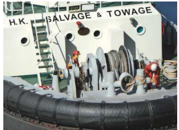
ABOVE: The foredeck area and ship-handling winch with two crewmen engaged in rope handling.
