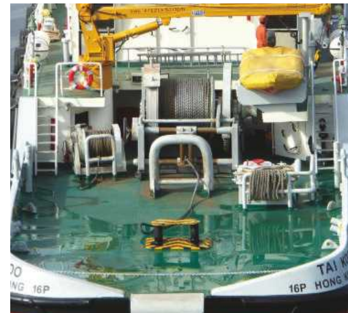
BELOW: Close-up of the stern towing deck showing the winches, deck crane, container lashing eyes, spare anchor and various stowed items.
